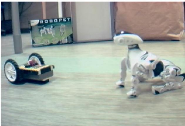
Figure 2. Controlling RoboPet from RCX using IR signals.
