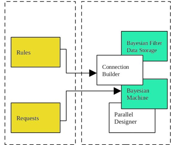
Fig. 3. Bayesian network simulator internal structure.
