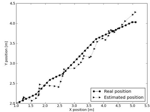
Fig. 8. Real and estimated path of the robot.
