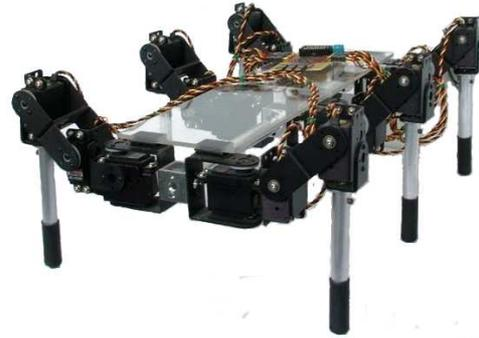
Figure 1. The hexapod — six-legged walking robot.
