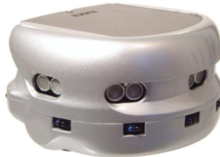
Figure 1. Mobile robot Khepera III
