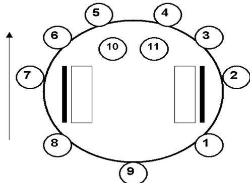
Figure 2. Position of the IR sensors
