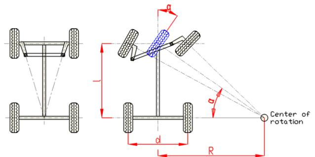
Figure 3. Ackermann steering principle
