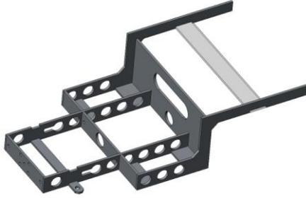
Figure 4. Front frame of the Bender II mobile robot
