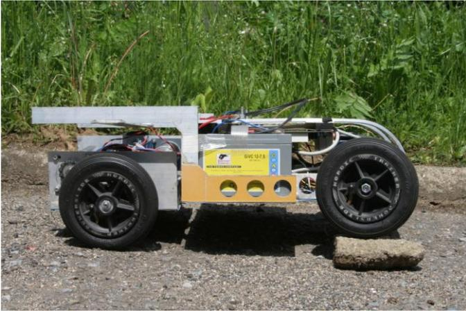
Figure 8. Swinging rear axle in action (side view)
