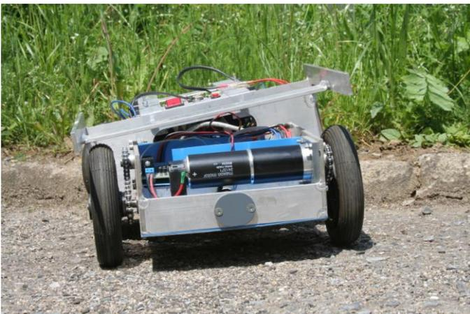
Figure 9. Swinging rear axle in action (rear view)
