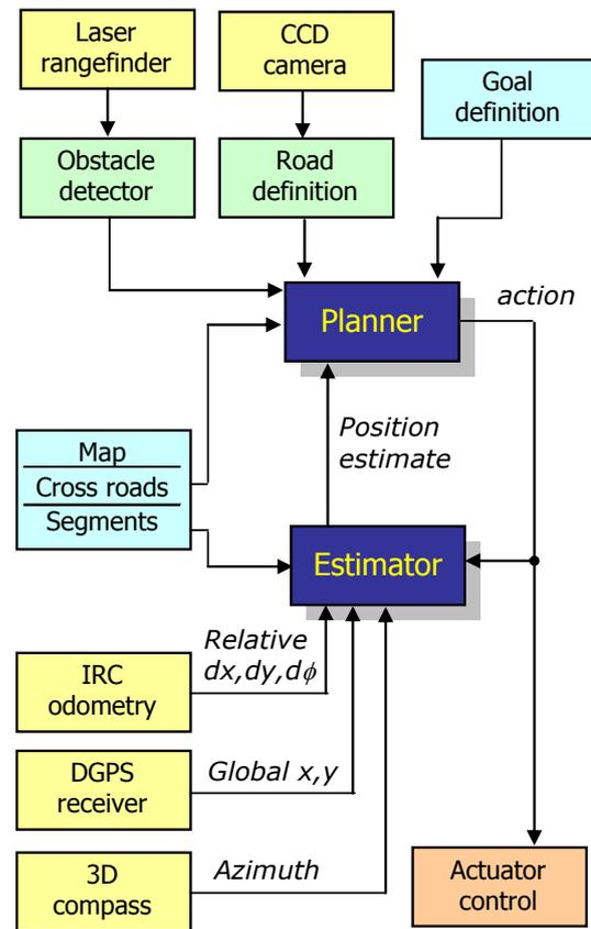
Figure 7. High level control scheme and signal flow
