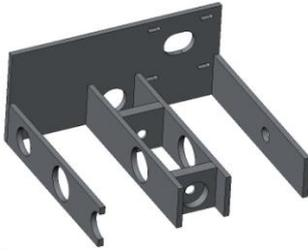
Figure 5. Rear frame of the Bender II mobile robot
