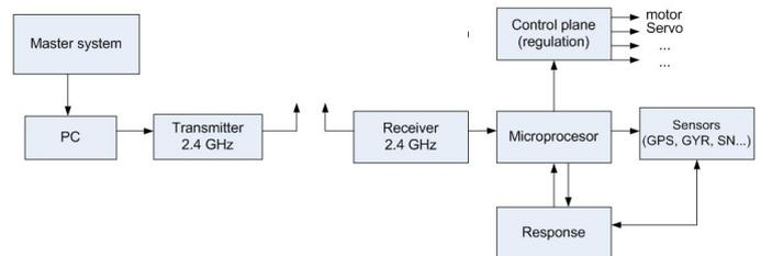
Figure 1. – the schem of the automatic autonomous system
