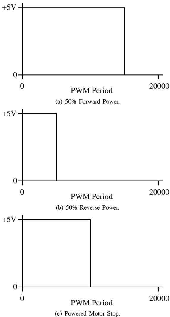
Fig. 1. PWM Motor Control with an H-Bridge.
