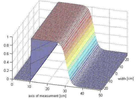
Figure 5. Infrared sensor in the occupancy grid.
