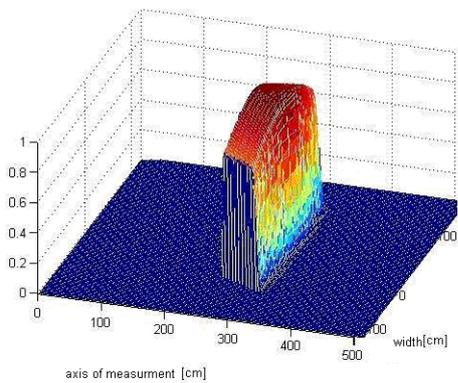
Figure 4. Uncertainty model of the ultrasonic sensor in the occupancy grid.
