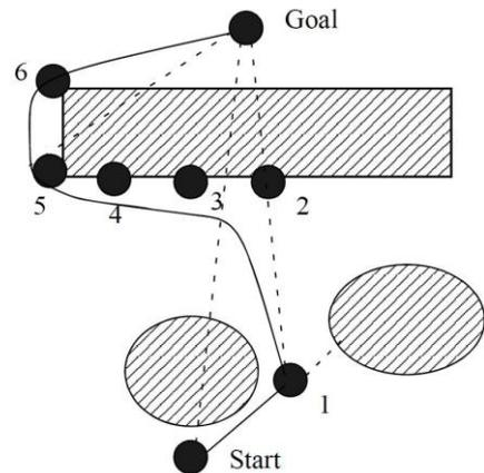
Figure 6. Principle of Wandering standpoint algorithm [4].
